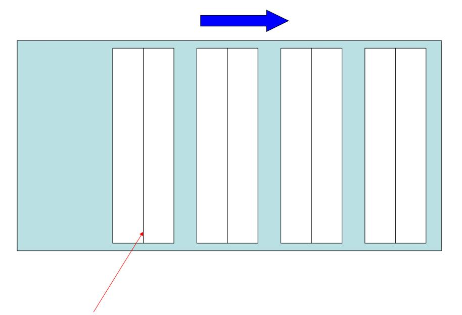
KISS-CUT: the top surface has been cut, but there is no gap between labels. When you remove the matrix during the manufacturing process, both labels keeps together and "seems like one" by the printer.
